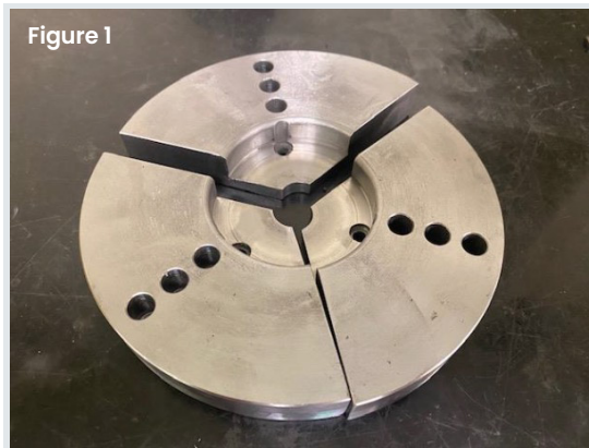
Figure 1 The original, heavy weight chuck design, produced by CNC.
